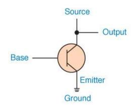
Figure 4.8 The connections of a transistor
