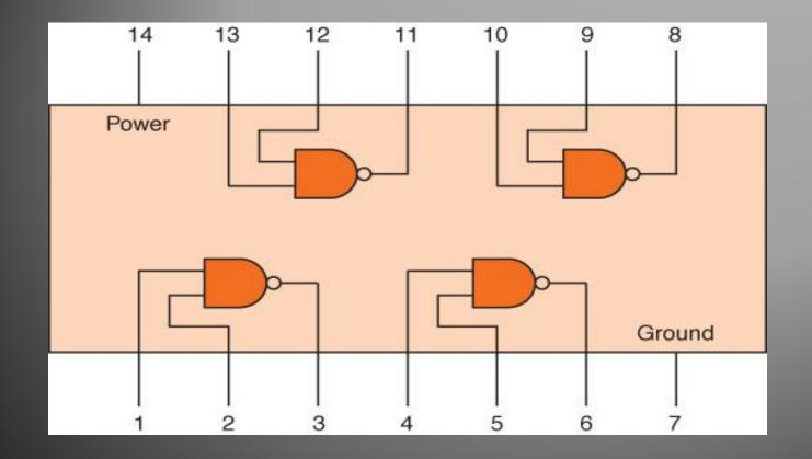
Figure 4.13 An SSI chip contains independent NAND gates
